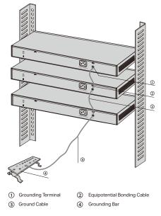
When equipotential bonding, please note that the cable should be copper wrapped Kelly with its area being 6mm<sup>2</sup> at least. The shorter cable the better, and use a grounding bar to establish an equipotential bonding point.
