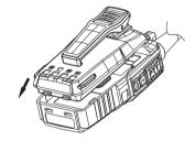
Press the top part of the battery towards the radio to lock it in place until a click is heard.
