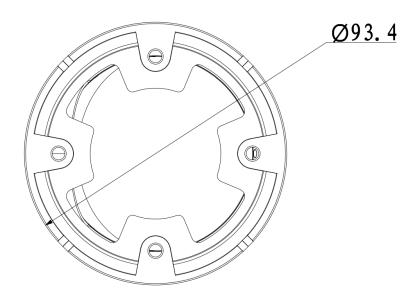
Figure 1-4 Dimension of Metal Dome 2
