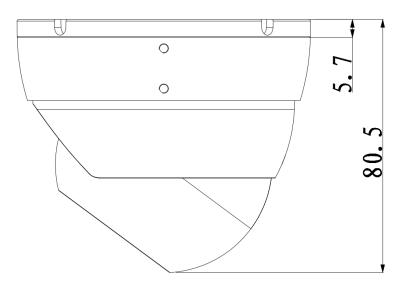
Figure 1-3 Dimension of Metal Dome 1
