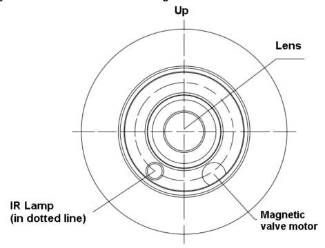
Figure 2-2 Device installation illustration 2
