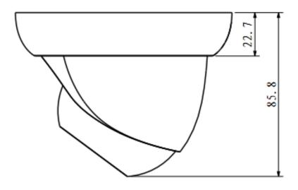
Figure 1-5 Dimension of Plastic Dome 1
