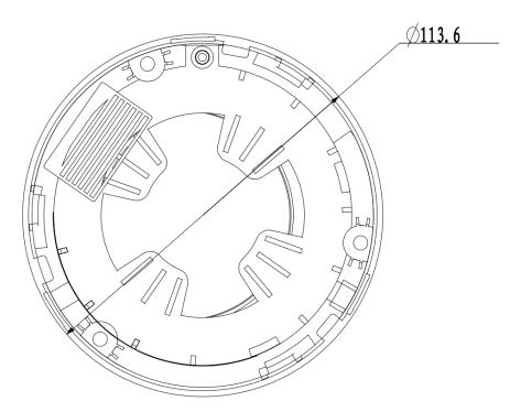
Figure 1-6 Dimension of Plastic Dome 2
