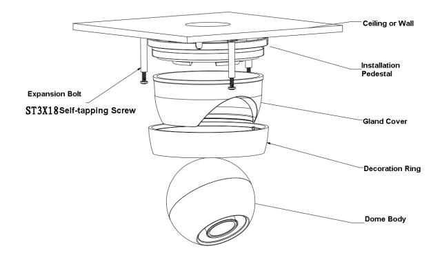
Figure 2-1 Device installation illustration 1
