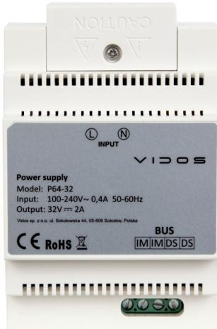
System Power Supply designed to operate in a two-wire digital system VIDOS 2IP, combining the functions of a power supply and voltage and signal separator.
