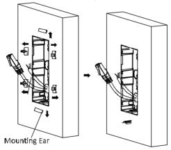
Figure 4-26 Remove the Mounting Ears
