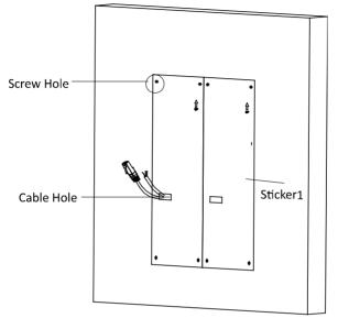
Figure 4-45 Chisel Screw Hole
