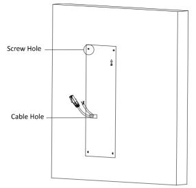
Figure 4-30 Chisel Screw Hole
