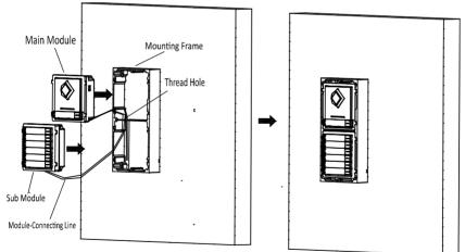
Figure 4-19 Insert the Modules
