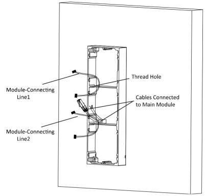
Figure 4-32 Placement of Lines
