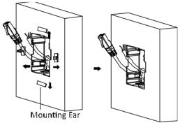
Figure 4-11 Remove the Mounting Ears
