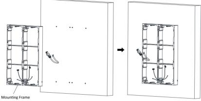
Figure 4-47 Fix the Mounting Frame
