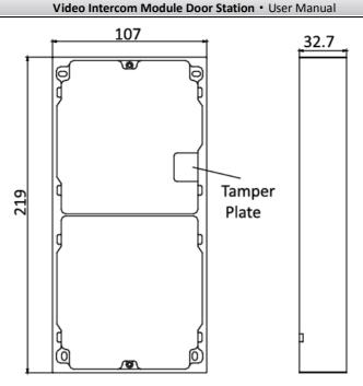
Figure 4-14 Front and Side View
