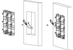
Figure 4-58 Mark the Screw Holes
