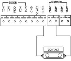
Door Magnetic Wiring Figure 3-4 Door Magnetic Wiring
