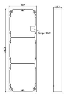
Figure 4-29 Front and Side View
