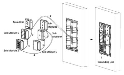
Figure 4-62 Install Mounting Frames
