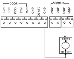
Figure 3-5 Exit Button Wiring
