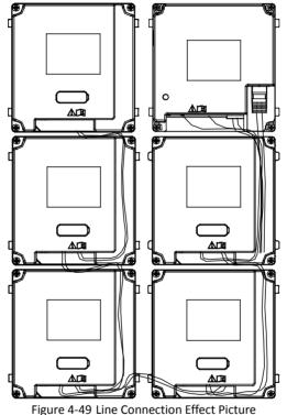
9. Insert the modules in to the frame after wiring. Main unit must be placed in the top grid on the left.
