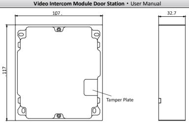
Figure 4-1 Front and Side View
