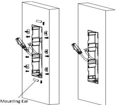
Figure 4-41 Remove the Mounting Ears
