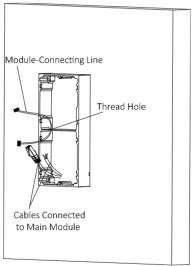
Figure 4-17 Placement of Lines
