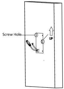
Figure 4-2 Chisel Screw Hole
