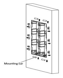
Figure 4-60 Remove the Mounting Ears
