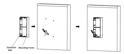
Figure 4-16 Fix the Mounting Frame
