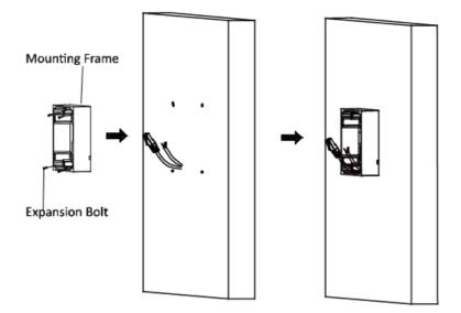
Figure 4-3 Fix the Mounting Frame
