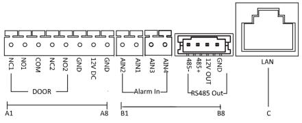
Figure 3-1 Terminals and Interfaces
