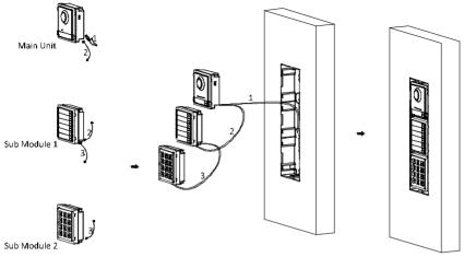
Figure 4-42 Connect Wires and Insert Modules
