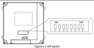
2. Set the sub module address according to the DIP rules, and install the rubber cover back.
