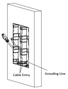
Figure 4-61 Place the Grounding Line
