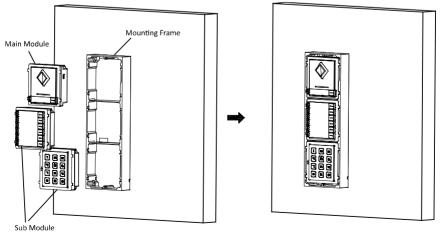
Figure 4-34 Insert the Modules
