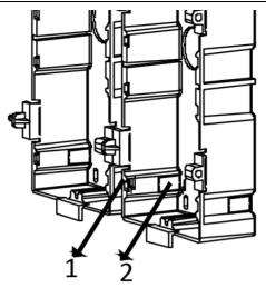
Figure 4-57 Remove the Plastic Sheets
