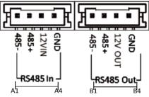
Figure 3-2 Terminals and Interfaces
