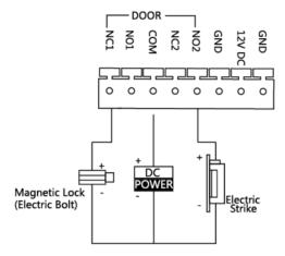
Figure 3-3 Door Lock Wiring
