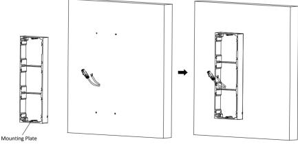
Figure 4-31 Fix the Mounting Frame
