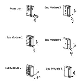
Figure 4-63 Install Mounting Frames
